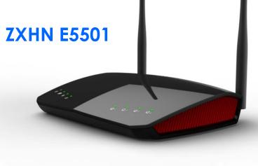
The E5501 is a wireless-N router designed for residential users that offers wireless speeds up to 300 Mbps. The E5501 has one Fast Ethernet interface for uplink and four Fast Ethernet interfaces for downlink.
